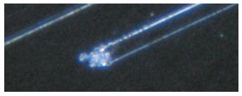
These scratches originated where a moving scraper encountered a fabricating debris defect. Scrapers do not scratch glass.
